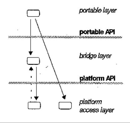
A system with a LAYERED ARCHITECTURE [B95a] is constructed as a number of linearly-ordered tiers, with the behaviour of objects in a given layer normally expressed in terms of the behaviour of objects in the same or lower layers. Objects in lower layers are often said to provide *services* to objects in higher layers.
