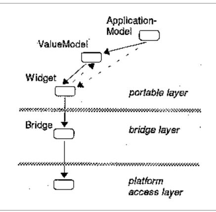
A bridge object is responsible for taking the native facilities of a particular platform and using them to implement the set of platform-independent capabilities which a particular type of Widget requires to implement its control in VisualWorks. So for example, a RadioButtonWidget would be furnished a Win32RadioButtonBridge on MS Windows, a MacRadioButtonBridge on the Macintosh and so on. Likewise, a ListWidget is matched with a Win32ListBridge, MacListBridge, etc., as appropriate.
